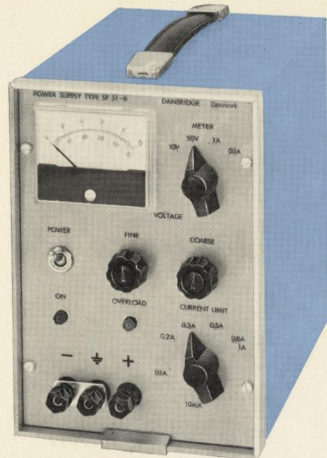
This power supply is fully transistorised and employs a controlled rectifier circuit for pre-regulation, thus reducing the power consumption and limiting the dissipation in the main regulating system.
